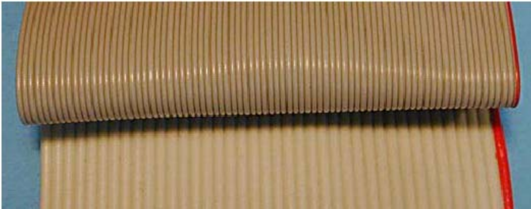
ATA/33 cable with 40 wires.
